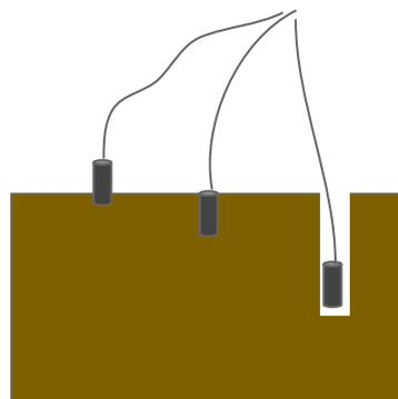
Vertical installation is less labour intensive and creates less ground disturbance than the horizontal installation; however, retrieval of the sensors for calibration and repair purposes can still be difficult. Typically in a vertical installation it is also more difficult to determine which soil horizon or features are present at the measurement depth, which may lead to uncertainty in soils with high spatial heterogeneity.
