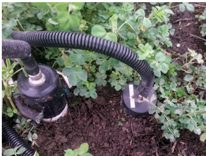
A vertically buried eosGP in an Alfalfa Field (Baldocchi Lab UC Berkeley)
