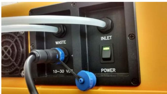
Figure 1. Attach the bare ends of the tubing to the INLET and WASTE ports on the UGGA.
