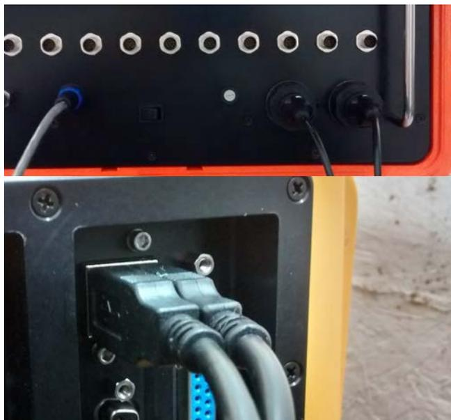
Figure 3. Attach the power and USB connections to the eosMX-P and plug the USB connections into the UGGA USB ports.
