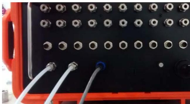
Figure 2. Attach the swaged ends of the tubing to the eosMX-P, and turn a further ¼ turn to secure.
