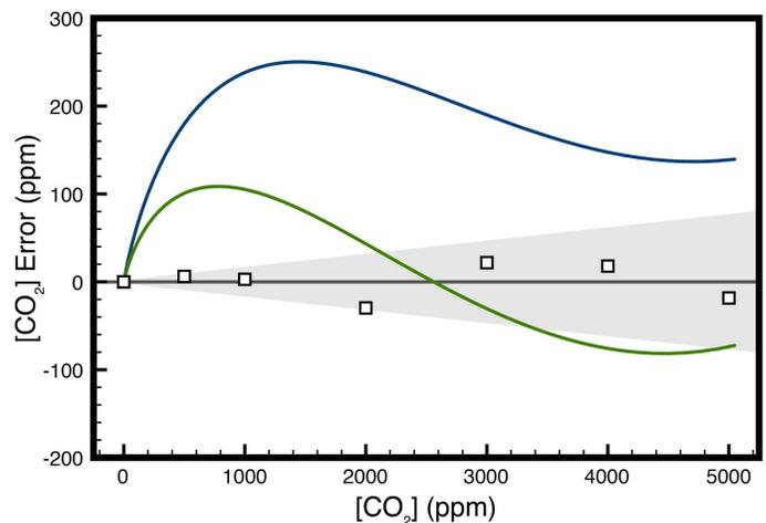
Figure 2. Error due to fitting 7 points spanning 0-50,000 ppm (blue), fitting 13 points spanning 0-50,000 ppm (green), and fitting 7 points spanning 0-5,000 ppm (open squares).
