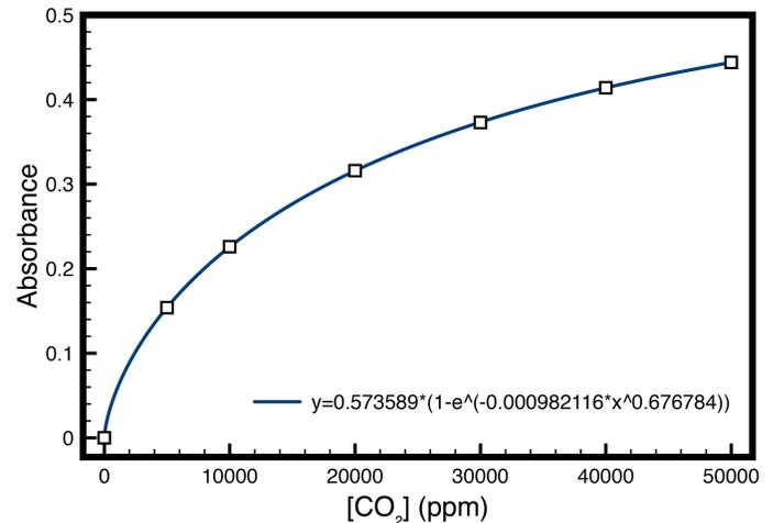
Figure 1. Best fit to a 7-point 0-50,000 ppm CO<sub>2</sub> calibration.
