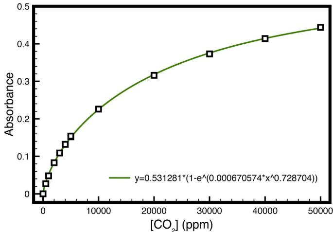
Figure 3. Best fit to a 13-point 0-50,000 ppm CO<sub>2</sub> calibration.
