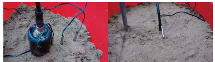
Figure 3. Left) Placement of radial thermistors. Right) Surface thermistor to measure ambient temperature.
