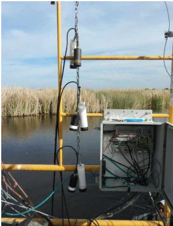
eosGPs connected to Campbell Scientific datalogger
